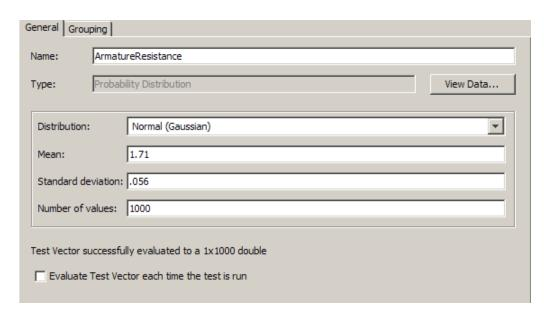
For this vector, the test is varying armature resistance up to a standard deviation of .056, around a mean of 1.71, and using 1000 values.
