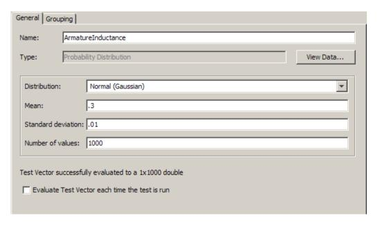
For this vector, the test is varying armature inductance up to a standard deviation of .01, around a mean of .3, and using 1000 values.
