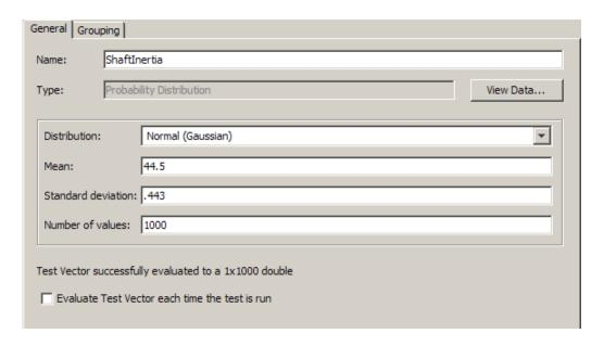
For this vector, the test is varying shaft inertia up to a standard deviation of .443, around a mean of 44.5, and using 1000 values.
