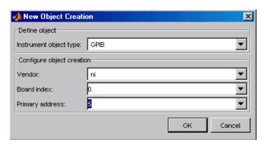
**9** Click **OK** to return to the Edit: Instrument1 dialog box, where the instrument object is now filled in and selected for this resource (GPIBO-5).
